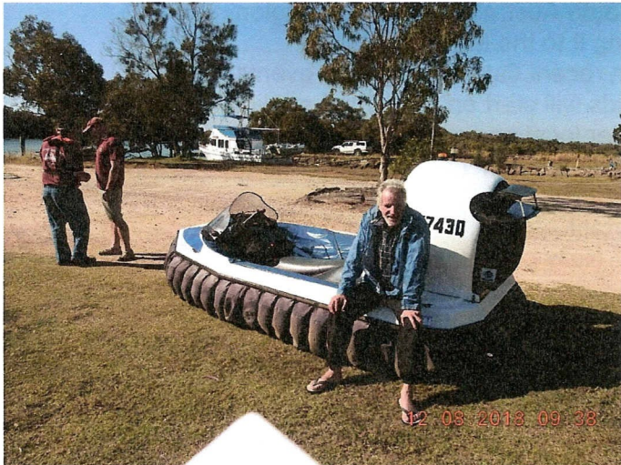
James & Elisha King towed their Revtech Renegade from Dundowran Beach for a display at the August boat show. 3.5m 20hp Honda GX690 900mm diameter Fan.
